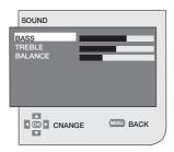
You can select the desired title to be processed from this menu. You can select the desired setting by pressing the **Up/ Down** movement buttons and adjust their levels with **Right/Left** movement buttons. You can adjust **BASS**, **TREBLE**, **BALANCE** levels as you desire. The changes you have made in the picture settings will be stored in the memory without requiring any other operations.
